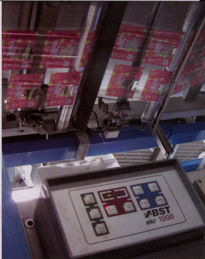
The Uteco Emerald press features an automatic viscosity control system, sleeves, and dual BST web guides.
