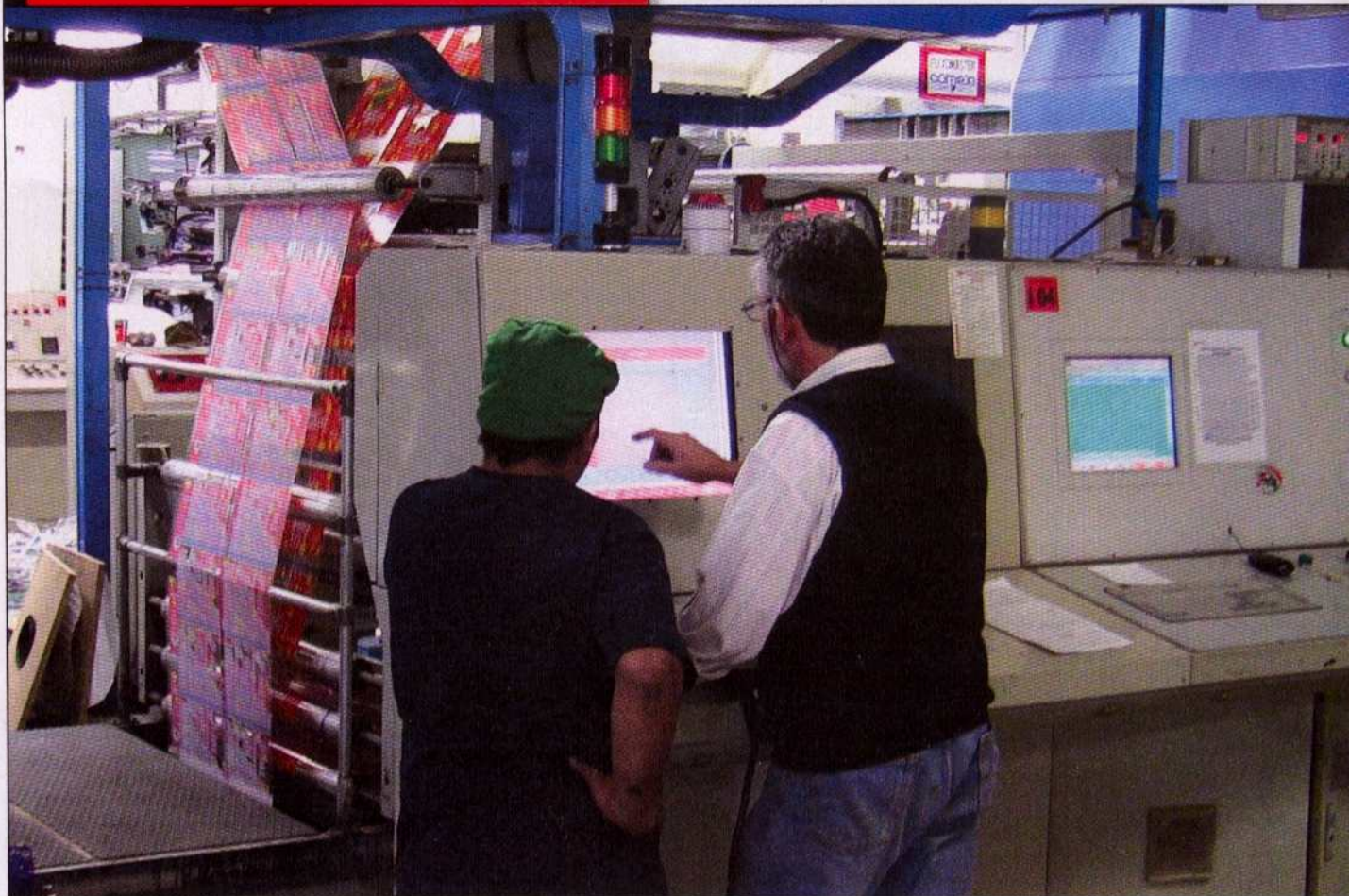
Victor Popoca and José Vicens use the Smart Register function on the BST Pro Mark print inspection system to set register with no special marks or plates.
